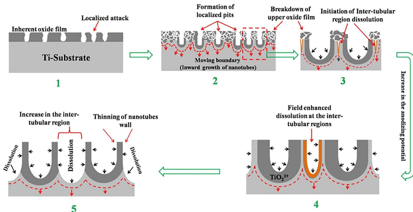
Fig. 5. Schematic representation of nanotubular growth as a function of the applied potential.
