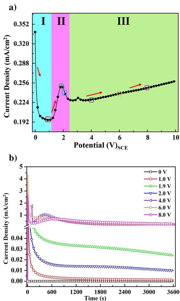
Fig. 1. (a) The LSV trend of cpTi-2 sample at 20 mV/s showing the current potential behavior in the anodizing electrolyte (b) The PSP trends showing the current response at OCP, 1, 1.9, 2, 4, 6 and 8 V (vs. SCE) constant potentials.
