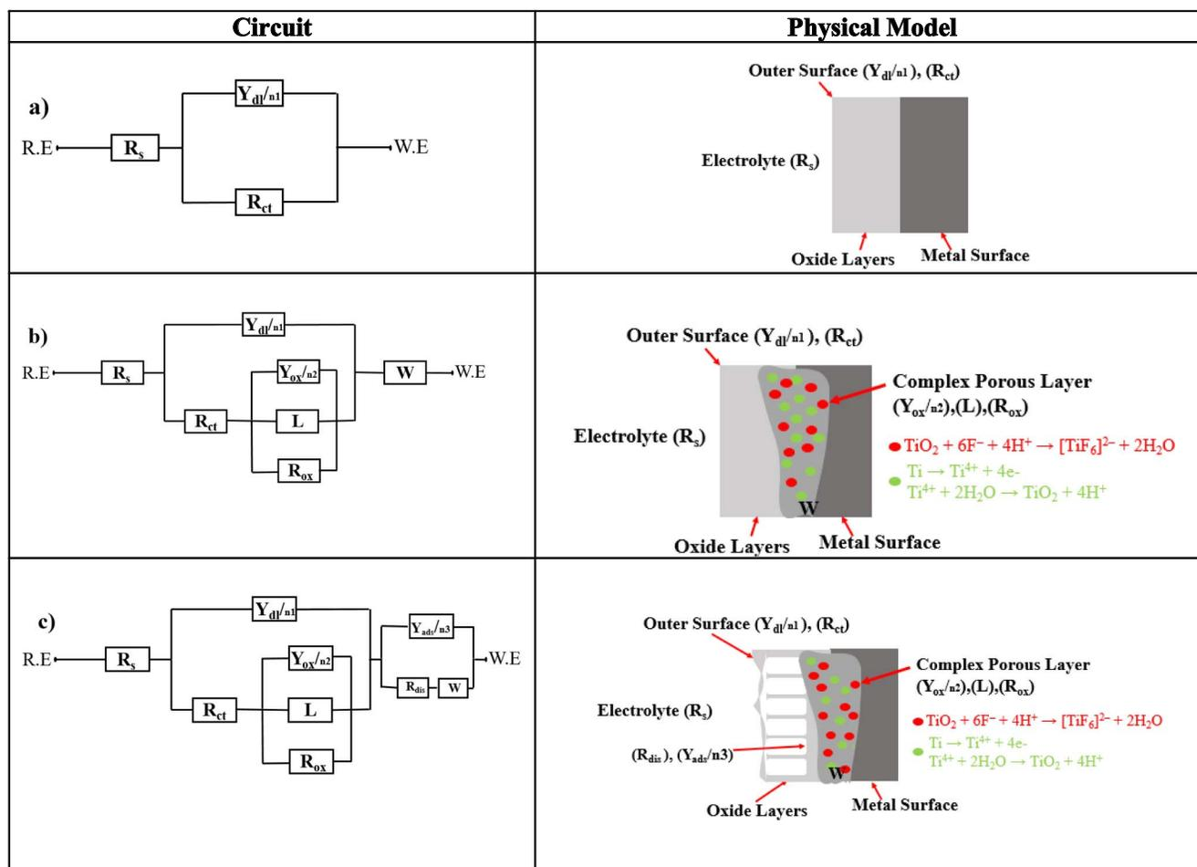
Fig. 6. Equivalent electrical circuit models used to simulate the impedance spectra with the interfacial electrochemical processes for (a) 0 V, 1 V (b) 1.9 V (c) 2, 4, 6 and 8 V.
