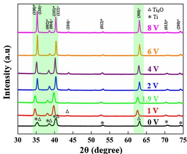
Fig. 3. XRD patterns of cpTi-2 anodized at various potentials. Note: The highlighted area shows the shifting of peak positions.
