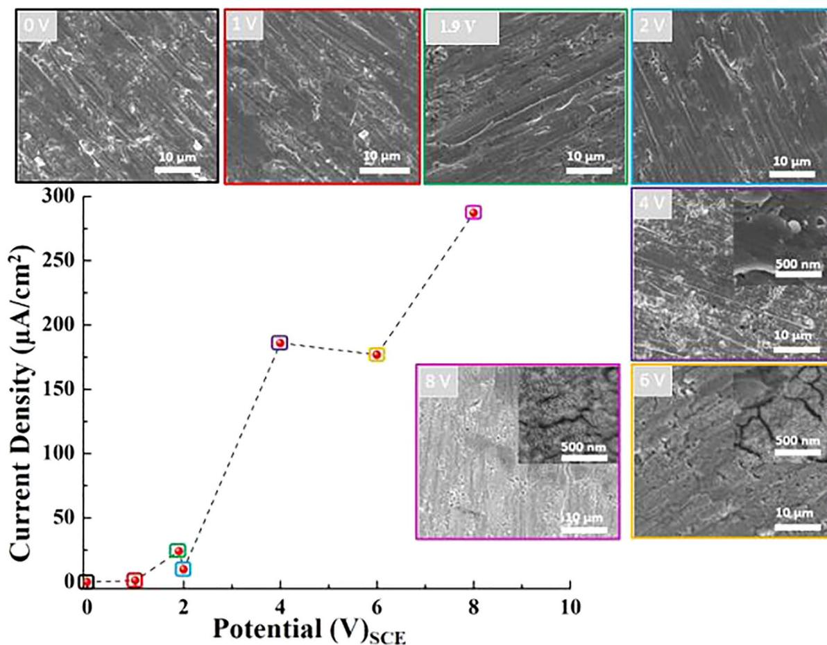
Fig. 2. The trend showing the current values obtained from PSP scans after 1 h polarization. The SEM images depicting the surface morphologies of cpTi-2 samples achieved after 1 h polarization at constant potentials.
