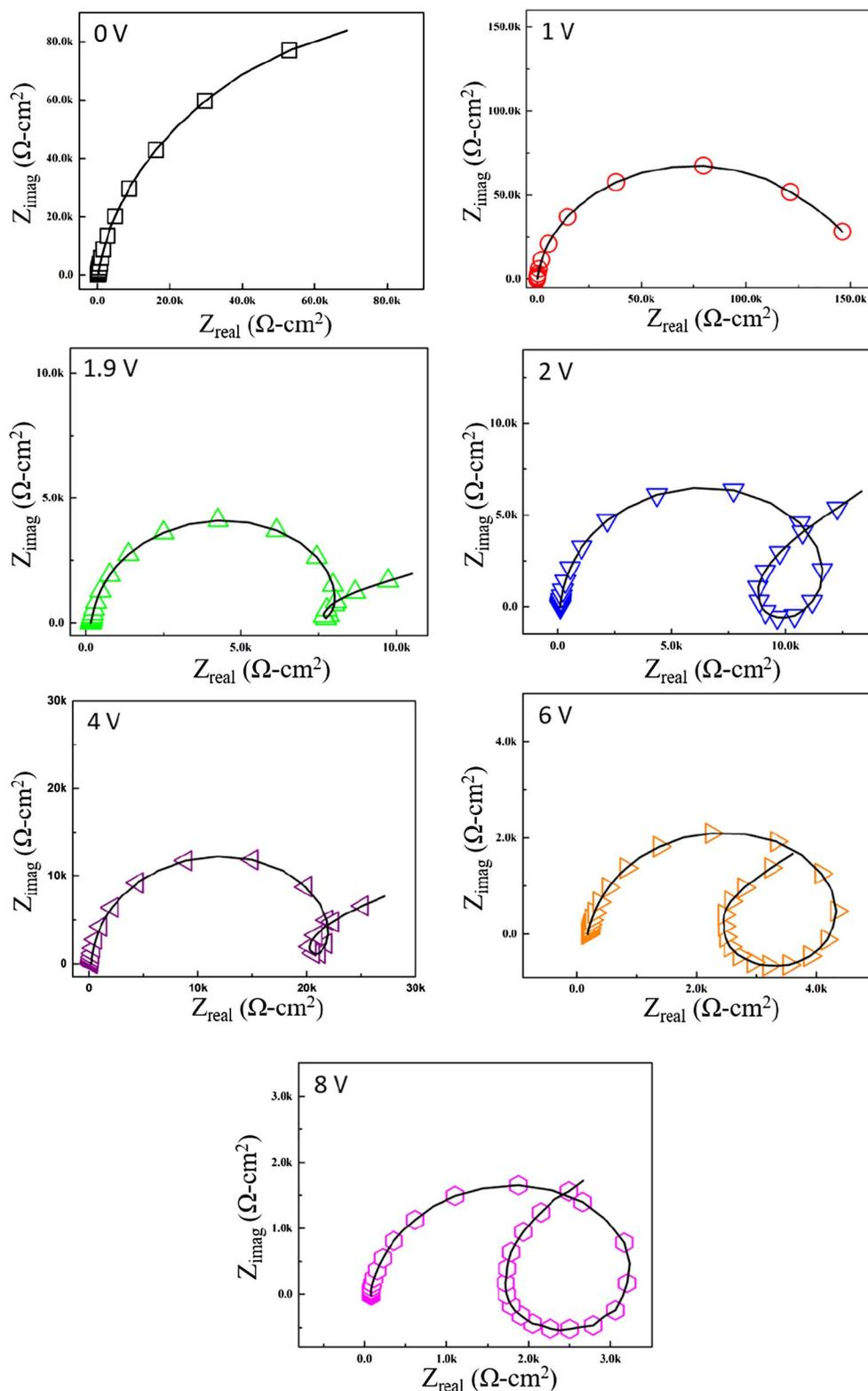
Fig. 4. The impedance spectra data points and fitted curves of cpTi-2 samples at OCP and various applied potentials ( $\leq 8$  V) in the anodizing solution.
