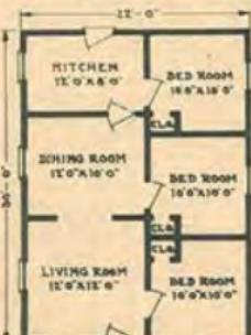
This plan gives slightly bigger rooms than Plan "A" by cutting out the bathroom. Makes a splendid plan where running water is not available.
