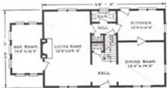
FIRST FLOOR PLAN
