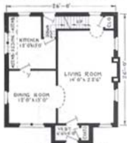
FIRST FLOOR PLAN No. 2
