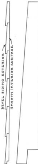
FULL SIZE DETAIL OF THE CLEAR AND KNOTLESS BEVEL DROP SIDING FURNISHED
