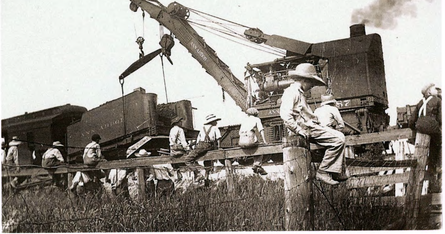
Photo #9: What a day for kids! A most unique photograph. The big Ann Arbor steam crane was probably brought up from Owosso. The job of lifting the heavy tender is underway. (In 2009 this crane in disrepair is on the grounds of the Buckley Steam Show site just west of Buckley MI in Grand Traverse County.)
