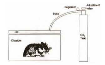
This calculated rate will allow a slow increase in the concentration of CO2 to develop. Without wind/hissing type noise in the chamber. You should NOT observe animals jumping, scratching at the sides of the chamber or rubbing their feet over their nose/mouth/eyes; if you do the volume is incorrect.
