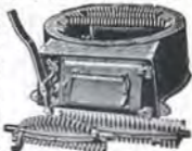
Grates and Ash Pit.
