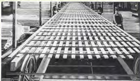
Largest conveyor of finished lumber in the world. It does the work of many men and horses.
