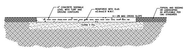
NOTE: CONCRETE PADS SHALL BE DIVIDED INTO UNIT AREAS OF NOT MORE THAN 30 SQUARE FEET AND NOT LESS THAN 16 SQUARE FEET, WITH CONTROL PLANE JOINT PROVIDE 100' MAX. EXPANSION JOINT SPACING. WHERE CURB DOES NOT EDGE WALK, DRAIN AWAY FROM BUILDING. EDGE PAD WITH 1" RADIUS AND BROOM FINISH SURFACE.
